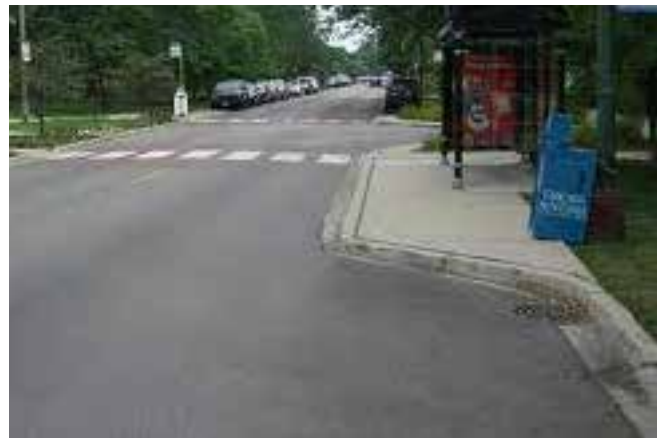
Curb extension or bulb-out
