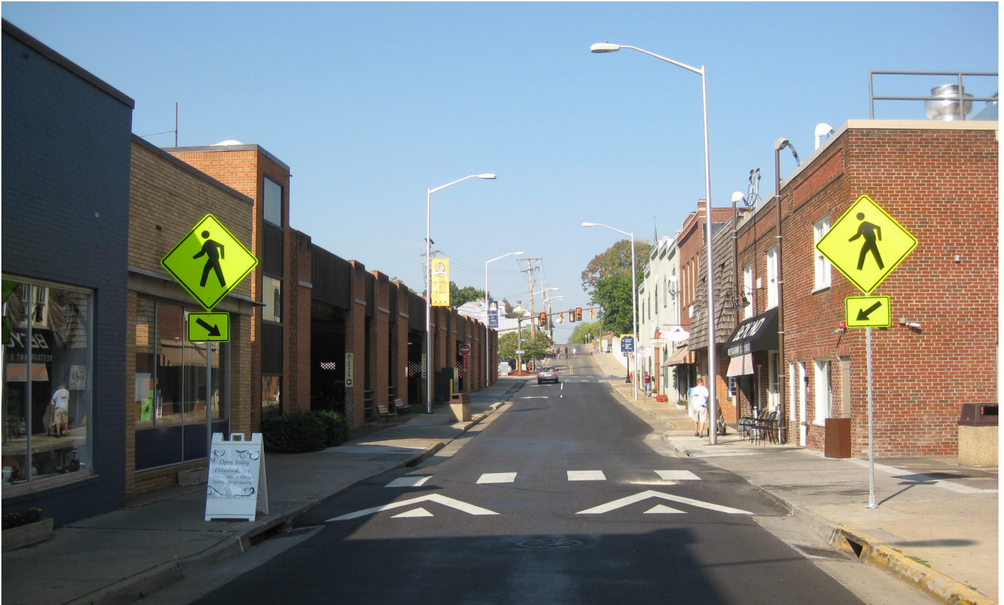
Raised crosswalk on Water Street, in downtown Harrisonburg, VA. Source: thanh.ha.dang, Flickr
